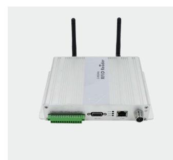
RS-AR01A fixed RFID reader operates in the 2.45 GHz band, with high recognition, long-range, powerful, high reliability& expandability and other characteristics, can work under extreme indoor and outdoor environment for different application.
